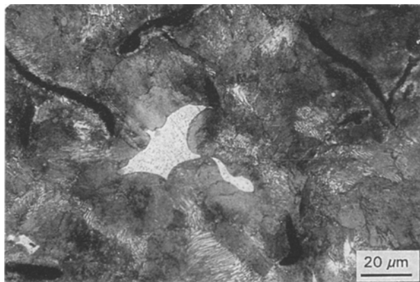
Figure 4 Photomicrograph of Alloy C specimen taken 25 mm from chill end and cast using a 25 mm chill.
