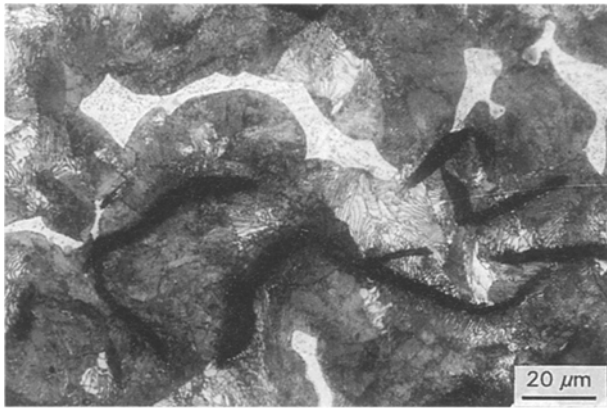
Figure 3 Photomicrograph of Alloy B specimen taken 25 mm from chill end and cast using a 25 mm chill.
