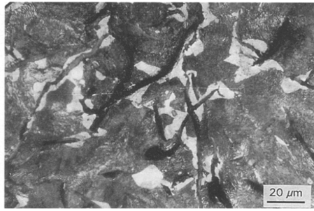
Figure 5 Photomicrograph of Alloy D specimen taken 25 mm from chill end and cast using a 25 mm chill.
